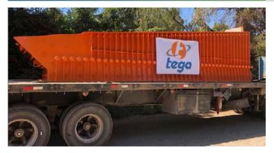
Wear resistant liners: Tega's aggression range comprises wear resistant liners used in transfer and storage equipment, handling bulk material in mineral processing and mining industries. The Company's wear-resistant liner products comprise D-MAC<sup>®</sup> Ceramic liners, Aggression rubber liner, Composite liner, Air blaster, Mosaic liner, Stallion-UNHWPME liner and Pro-line Polyurethane liner, Durotek<sup>®</sup> and Aggression Liner.
